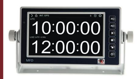
Devices communicate with each other through RS-232/RS-422 serial interfaces as well as Ethernet (PoE). As the primary data source, the master clock receives signals from external GPS receivers (NMEAO183 standard), as well as from built-in GPS receiver or internal real-time clock. If communication with the master clock is lost, the secondary clock seamlessly switches to the internal time signal source to maintain accurate timekeeping.
