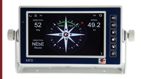
In the standard version, the MFD provides both numerical and graphic displays dedicated to the indications of the clock, GPS, gyrocompass, weather station, anemometer, log and echo sounder. At the customer's needs, it is possible to offer the presentation of other data, e.g. shaft rotation reading, steering column position and others. The MFD communicate with navigation devices over a NMEA0183 (RS-232/RS-422) or NMEA2000 - compatible with Canbus network and Ethernet (NMEA Over Ethernet).
