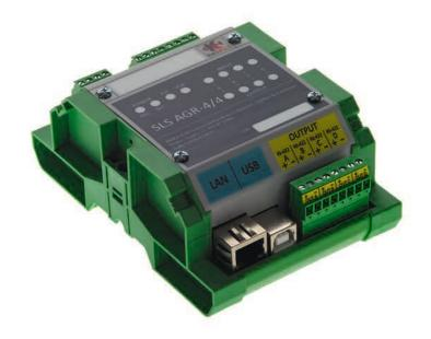
The SLS AGR-4/4 converter uses the standard short-circuit protected RS-422 ports to carry the NMEA 0183 data streams of up to the four input devices and four receivers. Each serial port can be set at one of the predefined data speeds - the device provides the data buffering when necessary.
